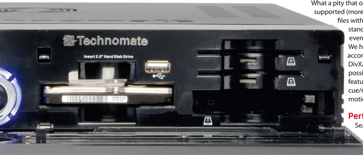
2.5in HDDs can be inserted into a slot behind the front flap
